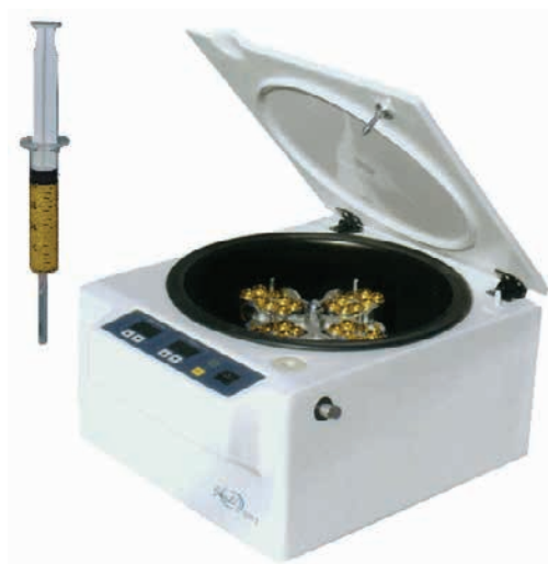
Fig. 10-4 Purifying the fat with a low-speed centrifugation machine. The speed should not exceed 1000 rpm.
